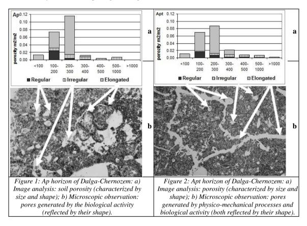
The image analysis data (Figure 1 a and 2 a) obtained for the total porosity in Dalga Chernozem showed that both soil horizons of the arable layer (Ap and Apt respectively) were moderately porous.
