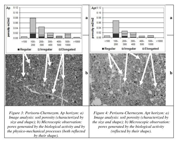
In this way, the image analysis data obtained for the pores grouped according to their type, showed that the transmission pores (50-500  $\mu$ m) are the most frequents in Ap horizon, while the fissures (> 500  $\mu$ m) had the highest values in the more compacted Apt horizon.
