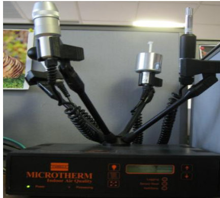
Figure 5 Casella MicroTherm (indoor climate system)
