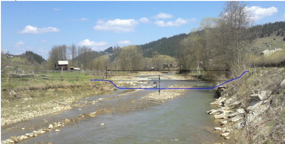
Figure 6: Upstream section for bankfull discharge determination
